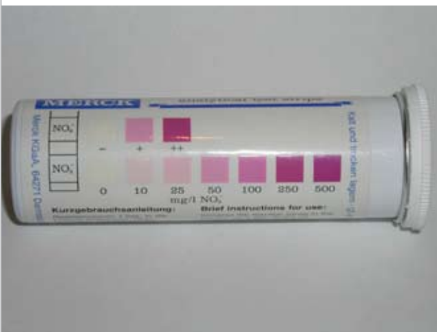
Nitrate test strips are cheap and water samples are quick to analyse (Photo WECF)
